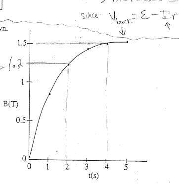
The data was obtained using a coil of 85 turns, having a cross-sectional area of  $4.0 \times 10^{-2} \text{ m}^2$ . The plane of the coil is perpendicular to the changing magnetic field (B). What is the magnitude of the average emf induced in the coil between t = 2.0 s and t = 4.0 s?
