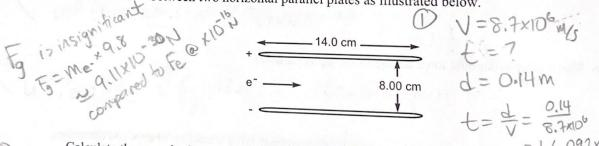
Calculate the magnitude of the vertical displacement of the electron as it travels between the plates.
