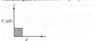
In the non-uniform electric field caused by a point charge, the electric potential energy can not be found as easily, but the reasoning is the same. Work done in moving a charged object in this non-uniform field is equal to the electrical potential energy gained and this is still the same as the area under the graph.
