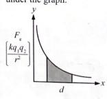
Using calculus, this area (the electrical potential energy) can be determined
