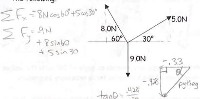
2. What is the magnitude and direction of the force needed to produce equilibrium with  $F_1$  and  $F_2$ ? apposite of net Fx and net Fy
