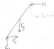
b) What minimum force of friction is needed at the base of the ladder to keep it from
