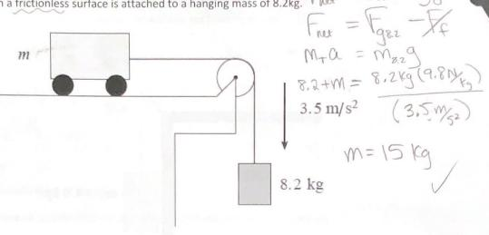
If this system accelerates at  $3.5 \text{m/s}^2$ , what is the mass m of the cart?
