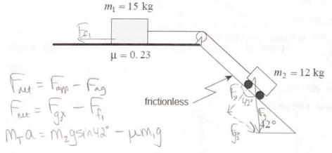
Determine the acceleration of the system of masses.
