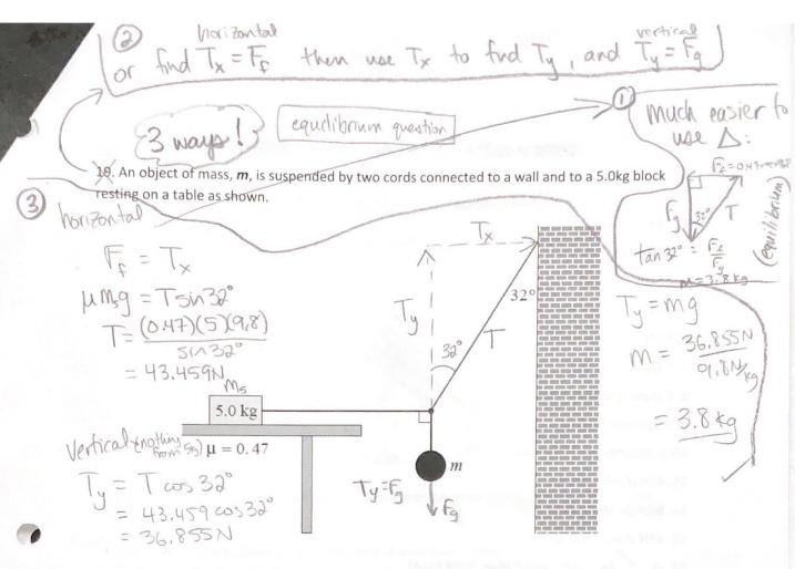
A coefficient of friction of 0.47 exists between the 5.0kg block and the table. What is the maximum mass, *m*, that can be hung from the cords before the 5.0kg block begins to move?
