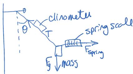
Measured  $F_{\text{spring}}$  at 5 different angles, see table
