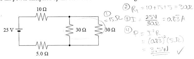
16. What is the terminal voltage of the battery in the circuit shown?
