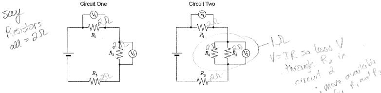
How have the values of V<sub>1</sub> and V<sub>2</sub> in circuit two changed compared to those in circuit one?
