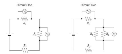
How have the values of V<sub>1</sub> and V<sub>2</sub> in circuit two changed compared to those in circuit one?
