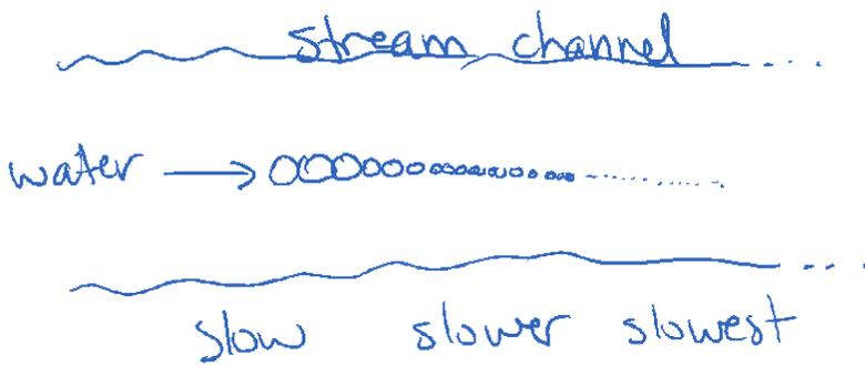
Stream particles are well sorted and rounded.
