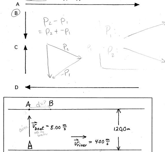
22. A motorboat starts from one side of the river, and aims directly across the river to point A. The velocity of the boat relative to the water is 8.00 m/s. The velocity of the river is 4.00 m/s, in a direction to the right on the diagram. The distance across the river is 120.0 m. The boat ends up landing at point B. How far down the bank from A is the actual landing point B?
