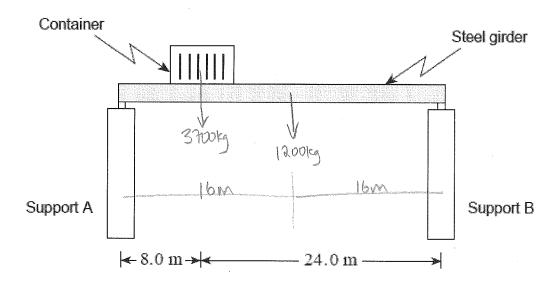
What are the upward forces at the girder end points when it is bearing a 3700kg shipping container 8.0m from support A?
