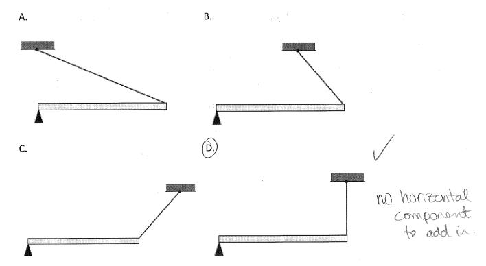
17. A crane is used to lift one end of a uniform 15m long pipe with a mass of 730kg as shown in the diagram below.
