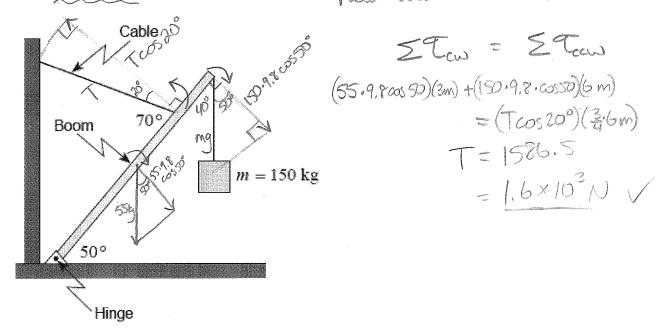
What is the tension in this cable when the boom when the boom supports a 150kg mass as shown?
