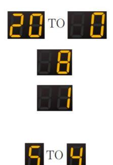
In counting down from 20 to 0, how many changes of state are there? In other words, determine the number of times segments are turned from unlit to lit plus the number of times segments are turned from lit to unlit. (Note that, in changing from 10 to 9, the left digit is turned completely off.)
