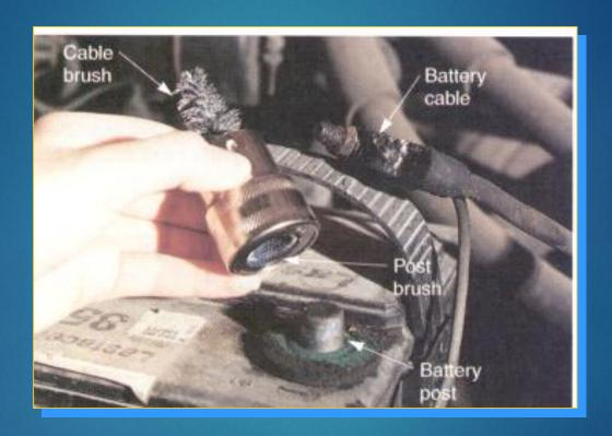
Use a post cleaning tool to remove **corrosion** from the posts and cable ends
