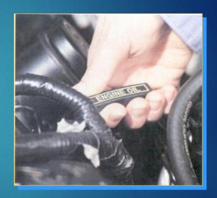
3. Wipe off the dipstick and replace it all the way into its tube
