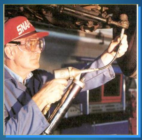
This technician is using a power **grease gun** to lubricate fittings
