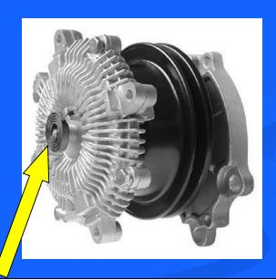
most belt driven fans have thermostatic clutches – these spin the fan only when the air temp thru the rad reaches a predetermined level
