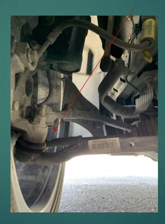
Tie rods, ball joints, and other bushings are clean without signs of wear, damage, or leaks
