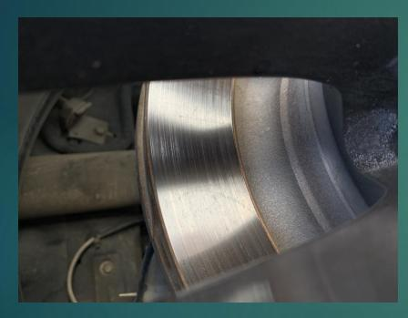
No cracks, grooves, or gouges
