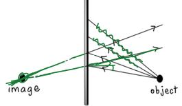
In a plane mirror, the image has the following characteristics:
