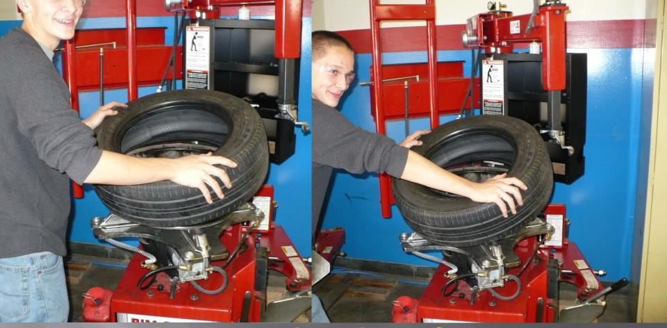
Lube Beads On Both Sides of Tire & Rim Before Re-Mounting, Place 'New' Tire on Rim and Push Lower Bead onto Rim Using Firm Hand-Pressure
