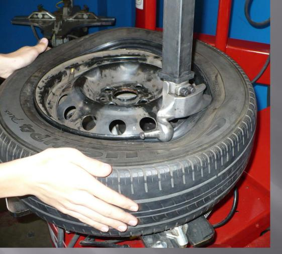
Press Down **On Table** "Rotate" Pedal, Assisting **Tire Under Bead While in** Rotation.
