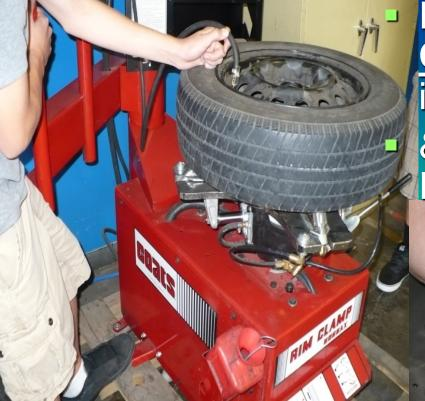
Remove hose and <u>QUICKLY</u> install the core into the valve stem. Check & Adjust Pressure as Required
