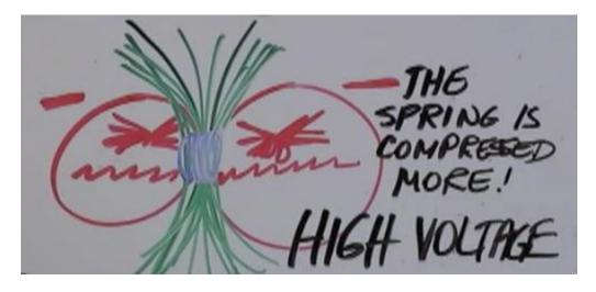
In this analogy, higher compression means higher voltage!
