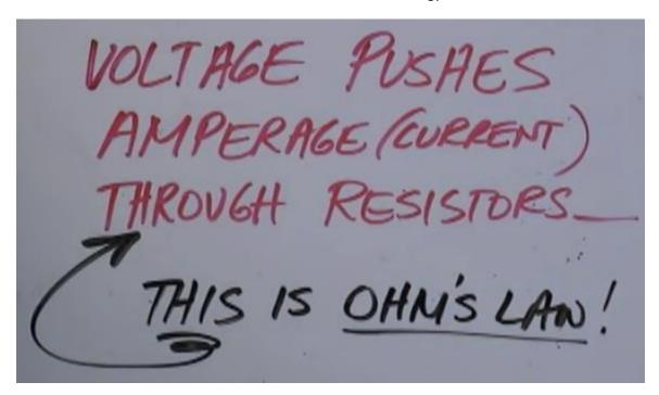
Voltage pushes amperage (current) through resistance!
